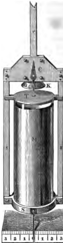
Fig. 62.—Mercurial Compensation Pendulum.
