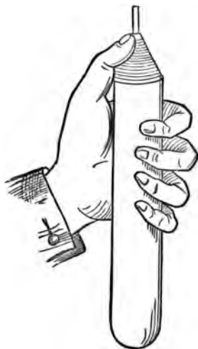
Fig. 42.—To polish Outer Sides of Coils.
